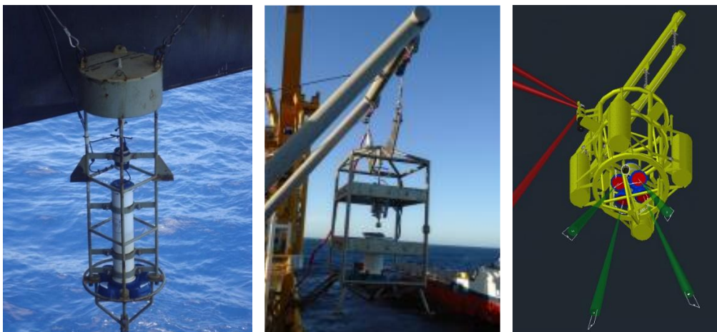
Figure 4: [left] cage model with ballast below [center] cage model with ballast integrated in the structure [right] 3D cage model showing acoustic signals propagating without obstacle.
